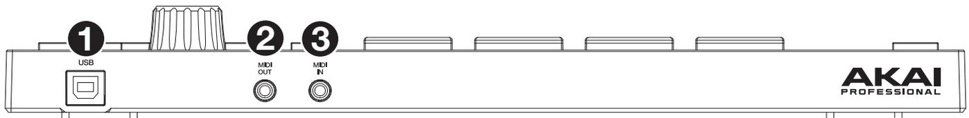
1. **USB-B Port:** Use the included USB cable to connect this high-retention-force USB port to an available USB port on your computer. This connection allows MPC Studio to send/receive MIDI data to/from the MPC software on your computer.
