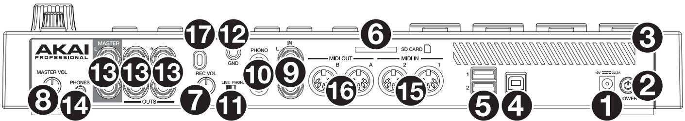
1. **Power Input:** Use the included power adapter to connect MPC Live to a power outlet.
