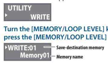
2. Turn the [MEMORY/LOOP LEVEL] knob to select "WRITE," and press the [MEMORY/LOOP LEVEL] knob.
