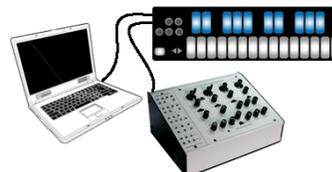
Use Case: In this scenario you can use an Expression Pedal (or any other uni-polar 0-5 Volt CV source) to control MIDI Software on the computer. Ableton Live will be used as the software example in this scenario but you can check for all the same things using different software.
