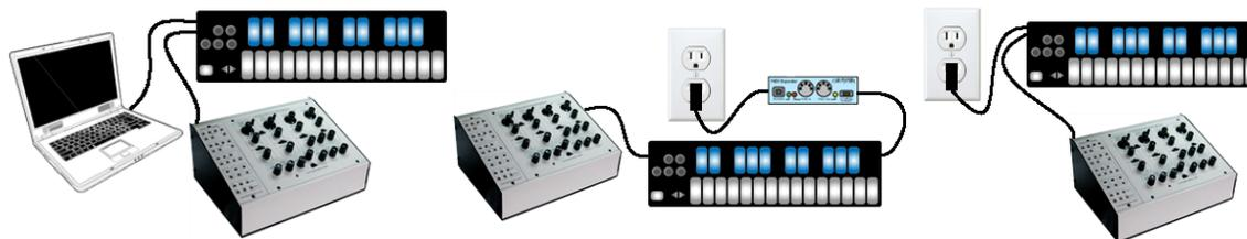
QuNexus can communicate with synthesizers or other CV devices using Control Voltages. Connect QuNexus to CV devices using a cable that is compatible with your CV device’s CV ports. Using adapters if needed, make sure one end can plug into one of the stereo 1/8in CV out ports on the left side of QuNexus. QuNexus’ CV input port (on the right side) requires one end to be a 3.5 mm TRRS (like the ones used for Apple iPhone headsets).
